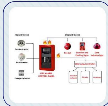
Fire Alarm Systems
